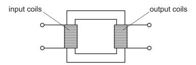
The output voltage needs to be lower than the input voltage.
